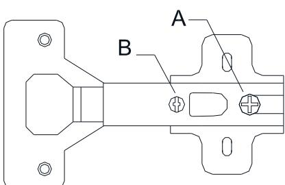
A = to connect the hinge to the door
