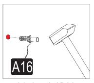
Attach the plugs to the drilled places.
